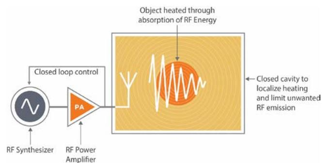
**Figure 3.** Solid-state powered RF energy application.
