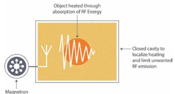
**Figure 2.** Magnetron-tube powered RF energy application.
