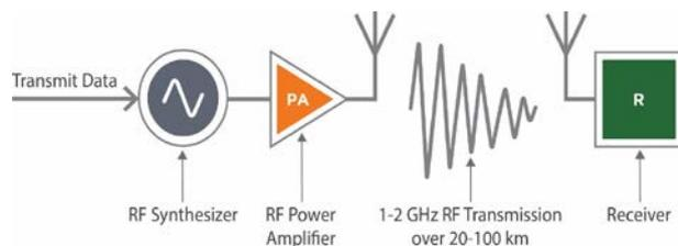
**Figure 1.** Typical RF data transmission block diagram.
