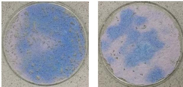
**Figure 2.** Colour changing desiccant identifying power distribution with (a) solid-state mode stirring enabled (left), and (b) no mode-stirring in a magnetron system (right). The Blue areas have had water boiled out of desiccant.
