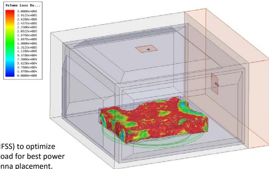
**Figure 1.** Using a simulator (HFSS) to optimize (for highest loss) a pan sized load for best power distribution by adjusting antenna placement.
