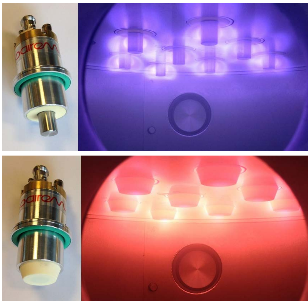
Figure 1. (a) Aura-Wave ECR microwave plasma source. (b) Multisource reactor consisting of 8 Aura-Wave units (shown in argon for a total microwave power of 160 W at 1 Pa). (c) Hi-Wave collisional microwave plasma source. (d) Multisource reactor consisting of 8 Hi-Wave units (shown in nitrogen for a total microwave power of 1600 W at 10 Pa).
