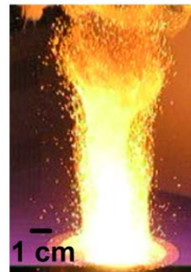
Figure 4. A flame ignited by solid-state LMH from thermite powder 10 .
