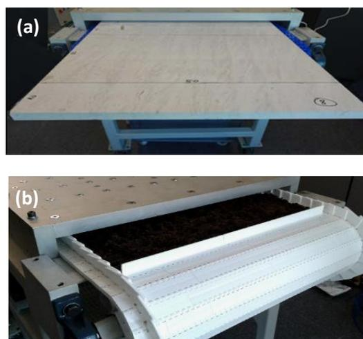
**Figure 2.** Examples of microwave applications (a) for flat materials, and (b) for granular materials with a conveyor belt for a cost-effective low temperature continuous flow.
