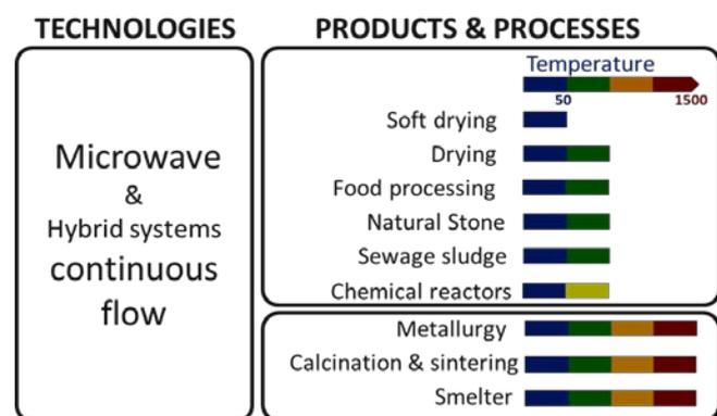
**Figure 1.** Proprietary technologies developed by CEINNMAT and partners, in different levels of implementation (at TRL 5-9).
