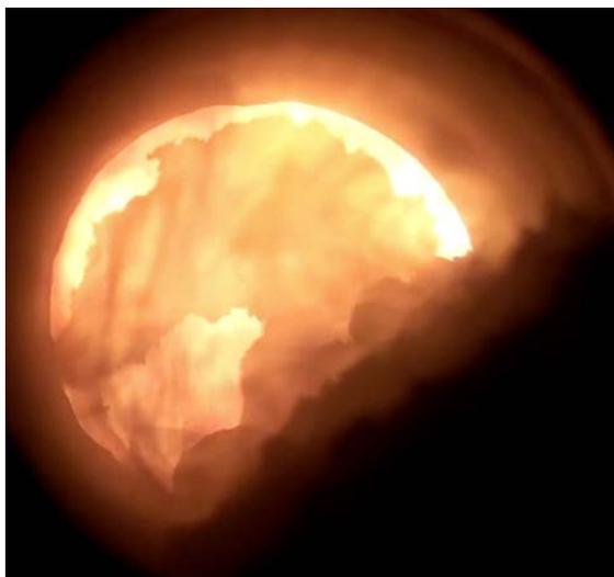
**Figure 5.** Rotary kiln interior during silicate calcination
