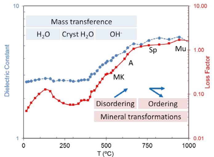
Figure 5. Microwave dielectric thermal analysis (MW-DETA). Dielectric constant (blue) and loss factor (red) vs. temperature during heating in a kaolinitic illite clay.
