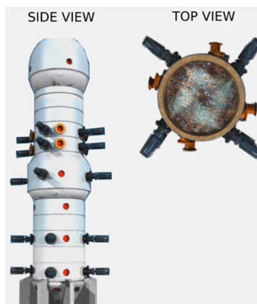
Figure 2. Schematic representation of multiple microwave generators attached to a single reactor 6 . Note that each of the black elements represents a 20 kW microwave plasmatron.
