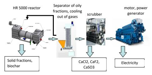
Figure 6. Installation for utilization of municipal waste with electricity production.
