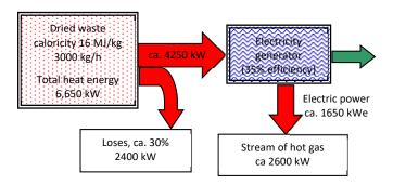
**Figure 8.** Energy balance for the system of microwave gasification of waste with caloricity of ~16 MJ/kg.
