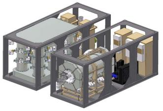
**Figure 10.** System for asbestos treatment installed within two standard containers.
