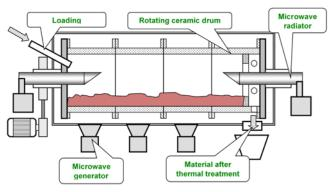
Figure 1. A schematic of the HR reactor.
