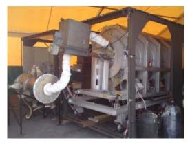
**Figure 2.** The HR-200 reactor installed inside a standard 20-feet container.
