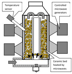
Figure 3. MOS construction scheme.
