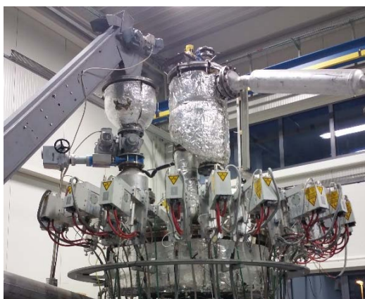
Figure 3: Microwave pyrolysis reactor (installed at Bionic Laboratories BLG GmbH, Germany, www.bionic-world.eu )
