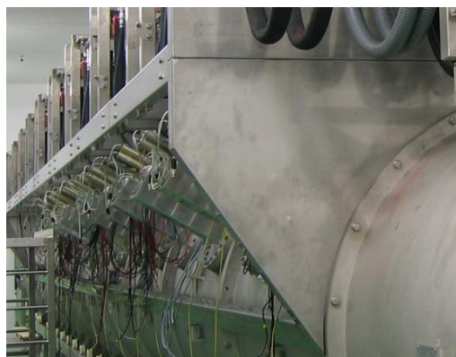
Figure 1: Microwave fruit dryer
