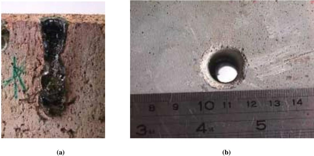
**Fig. 4. Microwave drilling in concrete: (a) A cut in an extensively radiated slab, and (b) a 13mm-diameter 10cm-depth hole made in a concrete slab by a cyclic microwave-drill operation.**
