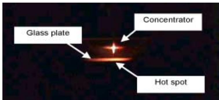
Fig. 3. Hot spot generated by the microwave drill in a glass plate.
