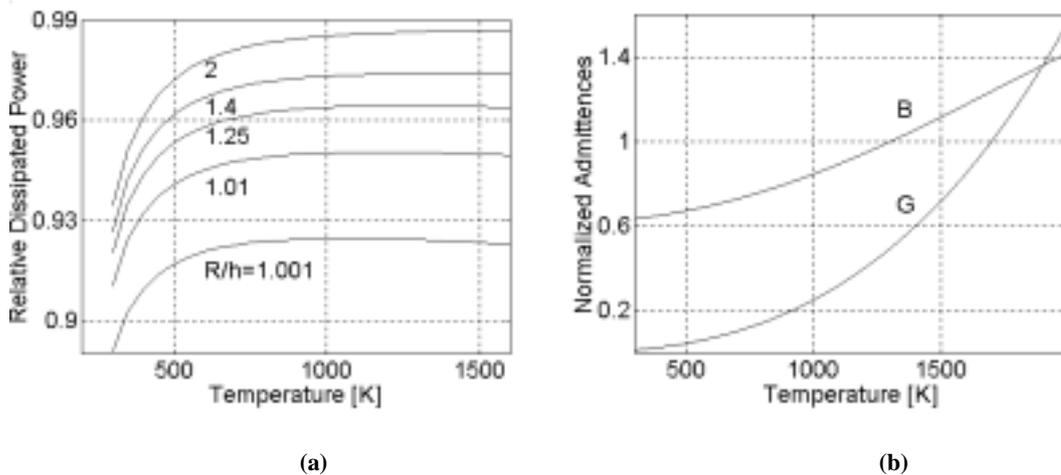
Fig. 5. Analytical calculations of the temperature dependence of (a) the relative absorbed power in spherical volumes of radius  $R$  around the antenna, and (b) the real and imaginary components of the monopole-antenna admittance ( $G$  and  $B$ , respectively). The material is pottery clay, and the monopole length is  $h=3\text{mm}$ .
