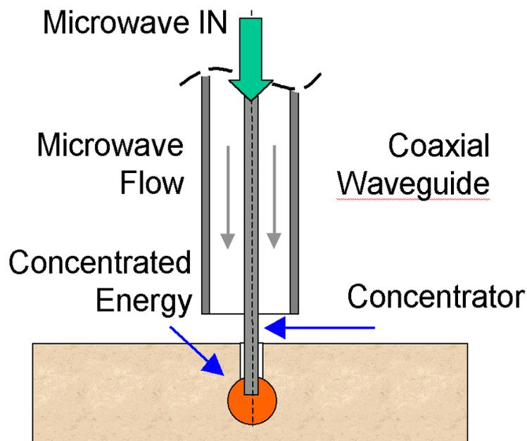
Fig. 1. A simplified principle scheme of the microwave drill.
