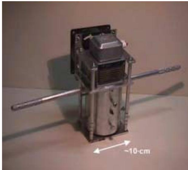
Fig. 2. The microwave-drill tool version.
