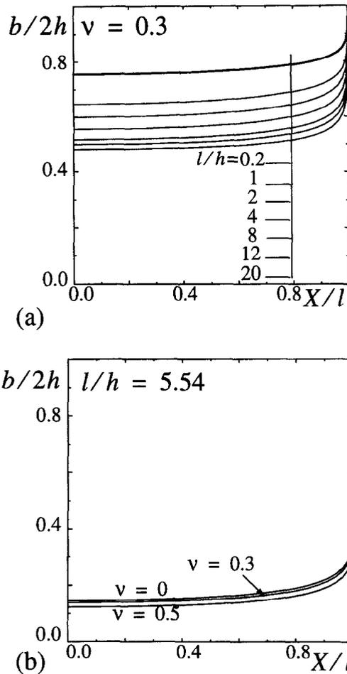
Fig. 6. Contact boundary versus the relative crack length: (a)  $l_f^0 = 2/3$ , various crack length to plate thickness ratio  $l/h$ ; (b) influence of the Poisson ratio, pure bending  $l_f^0 = \infty$ .
