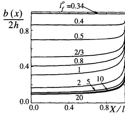
Fig. 4. Progression of the opening-closure borderline with an increasing remote load ratio;  $\nu = 0.3$ ,  $l/h = 10$ ; from top to the bottom  $l_f^0 = 0.34, 0.4, 0.5, 2/3, 0.8, 1, 2, 5, 10$ , and  $20$ .
