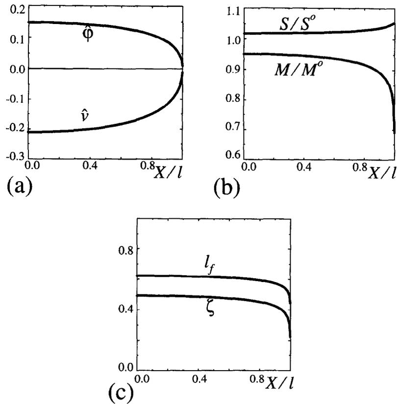
Fig. 3. Contact variable distribution versus  $\hat{x} = X/l$ ;  $l_f^0 = 2/3$ ,  $l/h = 10$ ,  $\nu = 0.3$ : (a) normalized in-plane displacement  $\hat{v}(X)$  and rotation  $\hat{\phi}(X)$ ; (b) the local contact induced in-plane force  $S(X)/S^0$  and bending moment  $M(X)/M^0$ ; (c) local load ratio  $l_f$  and relative through-the-thickness length of the crack  $\zeta$ .
