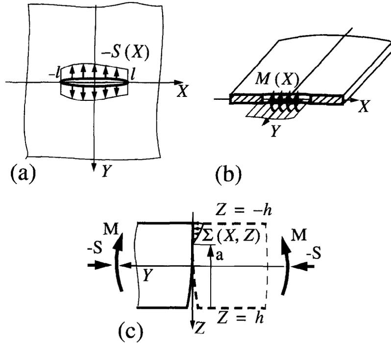
Fig. 2. Sub-problems: plane with a through crack under the action of a distributed (a) in-plane force and (b) bending moment; (c) edge-cracked strip subjected to extension and bending with closure.
