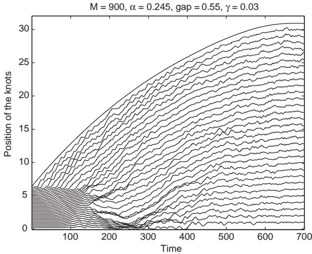
Fig. 13. Trajectories of the knots of the chain with waiting elements, impacted by the mass  $M_0 = 900$ . The chain sustains the extension. The model includes a small dissipation,  $\gamma = 0.03$ , the parameters of the constitutive function are  $\mu = 5$ ,  $\alpha = 0.245$ ,  $\mathcal{G} = 0.55$ .
