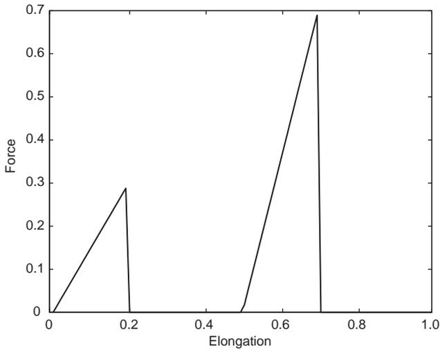
Fig. 8. Example of the constitutive relation corresponding to the links in the chain with waiting elements used in simulations. Shown constitutive relation is described by the following parameters:  $\mu = 5$ ,  $\alpha = 0.3$ ,  $\mathcal{G} = 0.25$ .
