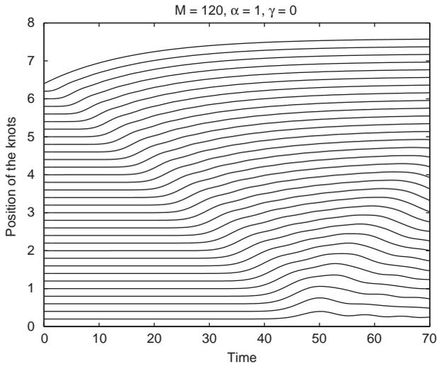
Fig. 5. The motion of the knots of the chain without waiting elements impacted by the mass  $M_0 = 120$ . The chain sustains the impact.
