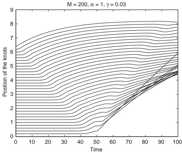
Fig. 11. With dissipation  $\gamma = 0.03$ , the chain without waiting links breaks being impacted by the mass of 200 units. The dissipation suppresses oscillations but does not prevent the chain from breaking.
