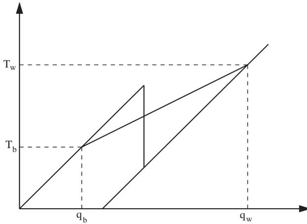
Fig. 4. Transition from one stable branch to the other occurs at the critical elongation  $q_b$ . The corresponding tensile force behind the transition front of the transition is  $T_b$ , the force ahead of the transition is  $T_w$ .
