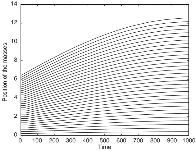
Fig. 14. With large dissipation,  $\gamma = 1$ , the chain impacted by a slow moving mass  $M = 70,000$  with the initial velocity 0.01. The chain sustains the impact; the dissipation suppresses the oscillations.
