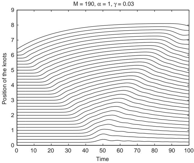
Fig. 10. The conventional chain without waiting links with small dissipation,  $\gamma = 0.03$ , sustains the impact of the mass of 190 units. The dissipation suppresses oscillations and allows the chain to support higher load.
