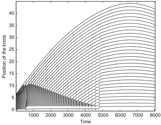
Fig. 16. Trajectories of the knots in the chain with waiting elements,  $\alpha = 0.3$ , and with a large dissipation,  $\gamma = 1$ , impacted by a slow moving mass  $M = 250,000$  with the initial velocity 0.01. The chain sustains the impact; the dissipation suppresses the oscillations. Observe the wave of partial breakage that propagates starting from the impact point. The closest to the root link experiences a partial damage because of the viscous-elastic wave.
