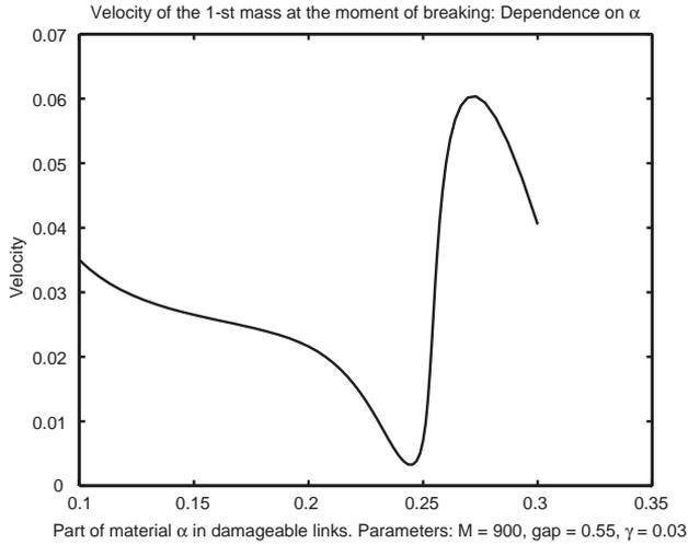
Fig. 12. Velocity of the large mass,  $M_0 = 900$ , at the moment of break of the chain for different values of the parameter  $\alpha$  modelling the fraction of the material in the basic damageable links. The model includes a small dissipation,  $\gamma = 0.03$ , the parameters of the constitutive function are  $\mu = 5$ ,  $\mathcal{G} = 0.55$ .
