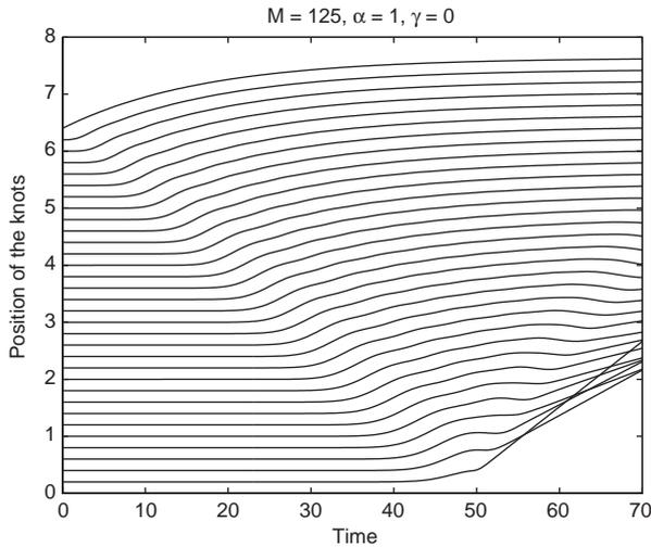
Fig. 6. The motion of the knots in the chain without waiting elements impacted by the mass  $M_0 = 125$ . The chain is broken. After the break, the bottom masses move up without resistance. However, possible collisions with neighboring masses are not taken into account in the calculations. As a result, the trajectories crossing occurs.
