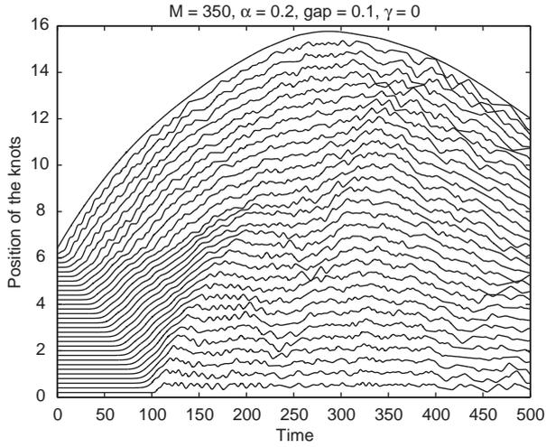
Fig. 7. Trajectories of the knots in the chain with waiting elements,  $\alpha = 0.2$ ,  $\mathcal{G} = 0.1$ , impacted by the mass  $M_0 = 350$ . The chain sustains the impact. Observe the elastic wave and two waves of a partial damage originated at both ends of the chain where the magnitude of the elastic wave is maximal. Notice intensive oscillations of the masses after all links are partially broken.
