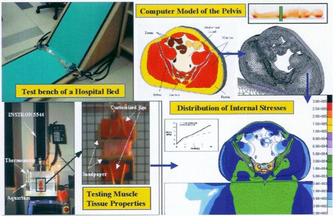
Internal stresses are calculated and displayed, based on data from a bed outfitted with standard pressure contact sensors, in an innovative TAU approach to preventing bedsores.
