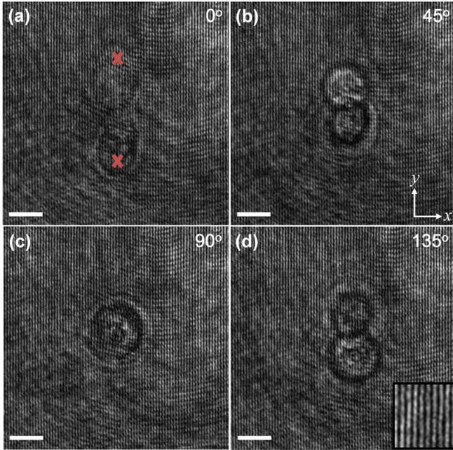
Fig. 2. Off-axis interferograms of yeast cells during  $180^\circ$  cell rotation obtained by HOTs, with  $5^\circ$  angular resolution. Examples for interferometric projections, taken at: (a)  $0^\circ$ , (b)  $45^\circ$ , (c)  $90^\circ$ , and (d)  $135^\circ$ . The inset in the bottom right shows a magnified area from the off-axis interference fringes at the background. The white scale bar represents  $5\ \mu\text{m}$  upon the sample.
