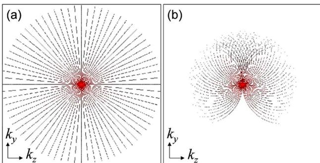
Fig. 3. Mapping of the  $k_y - k_z$  plane of the Fourier space derived from all projections, as based on (a) the back-projection method, and (b) the diffraction method.
