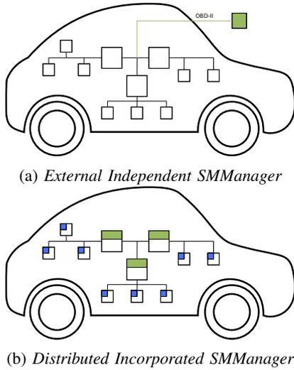
Fig. 4: *Safe-mode Manager* suggested topologies. The *SMManagers* are marked in green, while the *SMClients* are marked in blue. Note that Figure (a) shows one example for a system in *Transparent-mode*, while Figure (b) shows an example for a system in *Extended-mode*.
